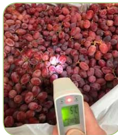
Measuring the surface temperature of Crimson Seedless table grapes with a handheld infrared digital sensor.
