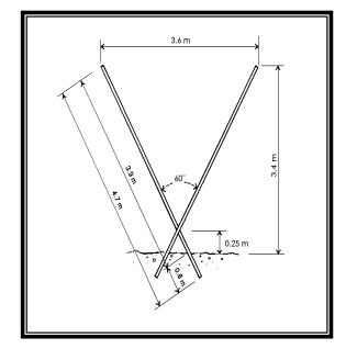
Figure 3: Basic configuration of Tatura Trellis.
